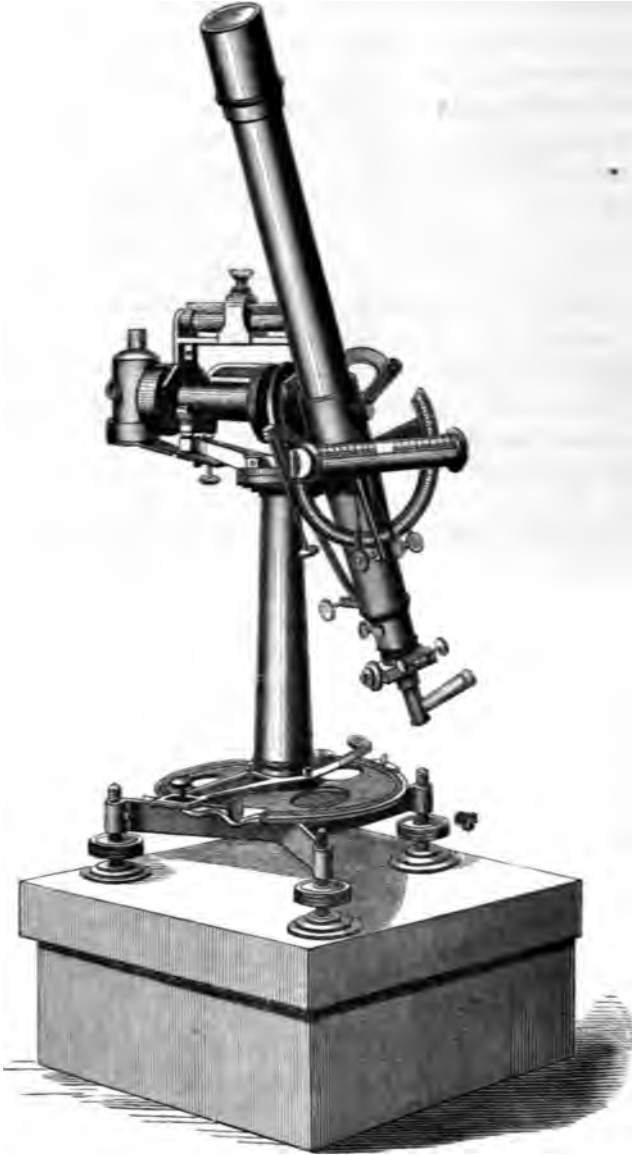
ZENITH TELESCOPE OF THE U. S. COAST SURVEY.
